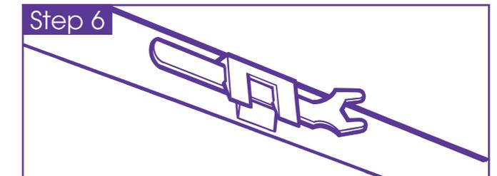
Step 6. Attach the spanner storage clip to the top of the door using the 1 x 15mm countersunk screw.
