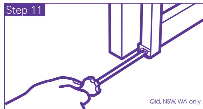
**Step 11** Fix the two nylon finger guides to the base of the frame using the elongated opening (for subsequent adjustment). The flexible portion protrudes into the cavity. When the guides are positioned correctly, fasten with a 15mm round head fixing screw.
