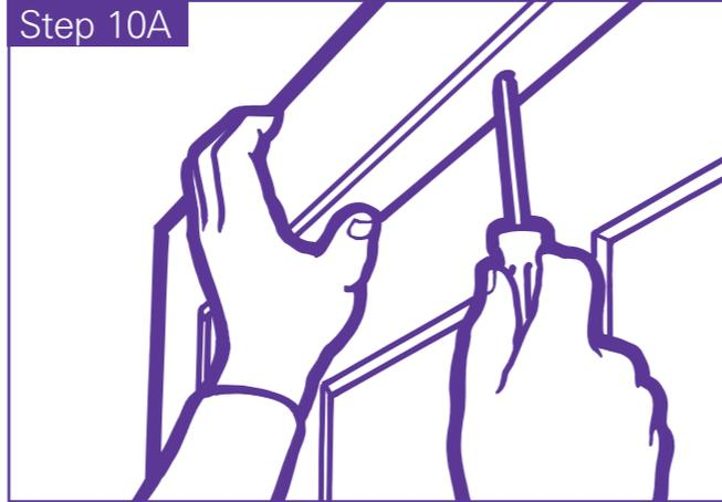
**Step 10A** Screw in place the removable fillet using 4 x 35mm screws through a white snap cap base. Finish off with supplied snap caps. Refer to Steps 10A, 10B and 10C.
