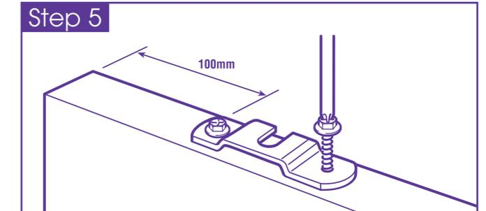
Step 5. Attach the door support brackets to the top of the door using the 4 x 30mm hex head screws, 100mm in from each side.
