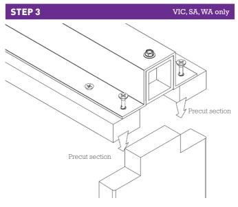
Cut down the sides from the end of the closing jamb – refer to the pre cut section in the detail shown. Screw (not provided with fittings) the closing jamb to the head section fixing through the head timber into the closing jamb stile.
