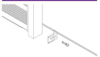
Fix the two nylon finger guides to the base of the frame using the elongated opening (for subsequent adjustment). The flexible portion protrudes into the cavity. When the guides are positioned correctly, fasten with 2 x 15mm round head screws.
