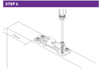
Attach the 2 x door plates to the top of the door using the 8 x 38mm hex head screws. The door plates are fixed 75mm in from each side and central to the thickness of the door. **Ensure both door plates are facing in the same direction**
