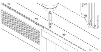
Fit and screw the head track assembly to the cavity pocket using the 10 x 16mm button head metal thread screws. **Do not remove the temporary throat spacers in the opening of the cavity throat until the wall sheeting has been completed. Failure to adhere will void warranty.**
