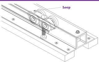
Place 2 x carriage assemblies in the track. Ensure side of roller with "Loop", is inserted first.
