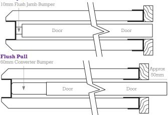
**Please note:** For a flush jamb fitment, install the 2 x 10mm converter bumper stops onto the edge of the door, closest to the cavity pocket. To convert a flush jamb cavity into a flush pull unit, install the 60mm converter bumper stop onto the edge of the door, closest to the cavity pocket and central to the height of the door. Ensure the position of the bumpers are not in line with the backpost fixing screws. Some unit sizes/ types may not be available in all states.
