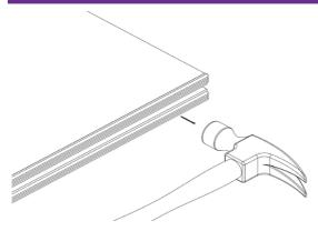
Cut the 2 x glide guide strips to suit the door width. Tack both strips to the bottom of the door using 5 x panel pins with each glide guide strip. (Total 10 x panel pins).
