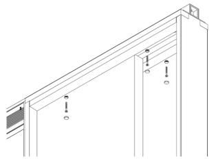
Screw in place the removable fillets using 4 x 35mm countersunk screws through a white snap cap base. Finish off with supplied snap caps. Refer to drawing in step 11 and diagram 11A or 11B depending on your state.
