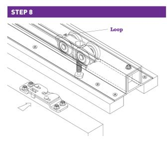
With the door in the cavity opening, lift the door to locate each door plate onto the carriage assembly bolt..
